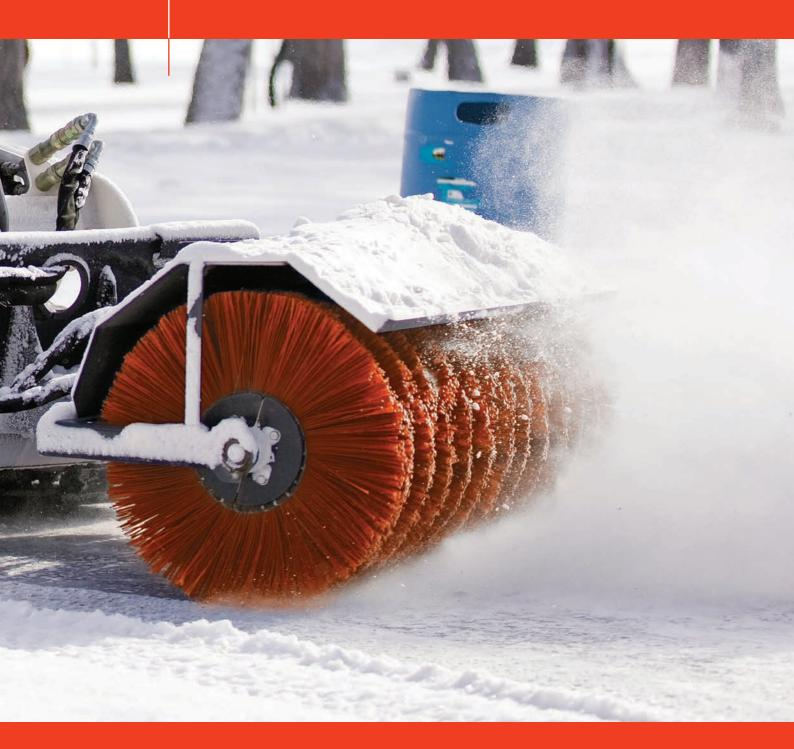
A wide range of bristles, covering Bobcat<sup>®</sup> and other brands of attachments, lets you make a clean sweep of debris such as asphalt, clay, gravel, light snow and sand.
